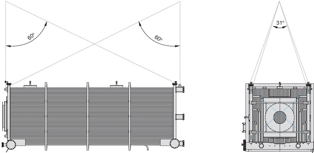
Firebox slinging. Change of transport position to operating position by means of two cranes (in order to avoid dragging)
